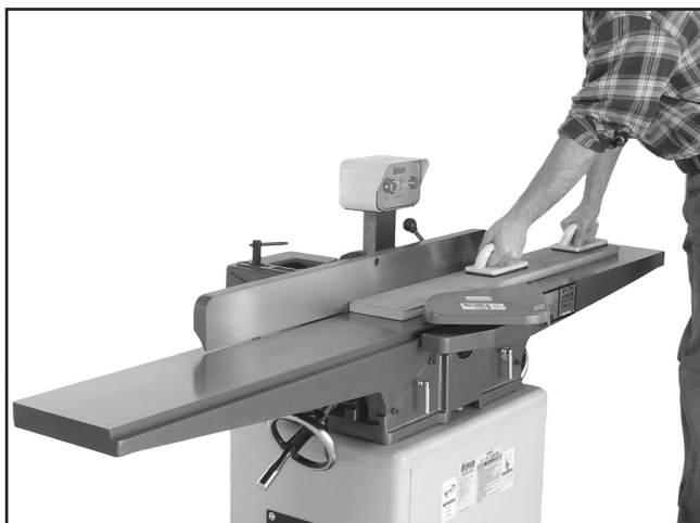
Figure 22. Typical surface planing operation.
